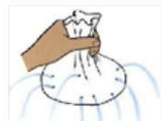
Fig. 8.9 Transmission of pressure in the water in a closed polythene bag
