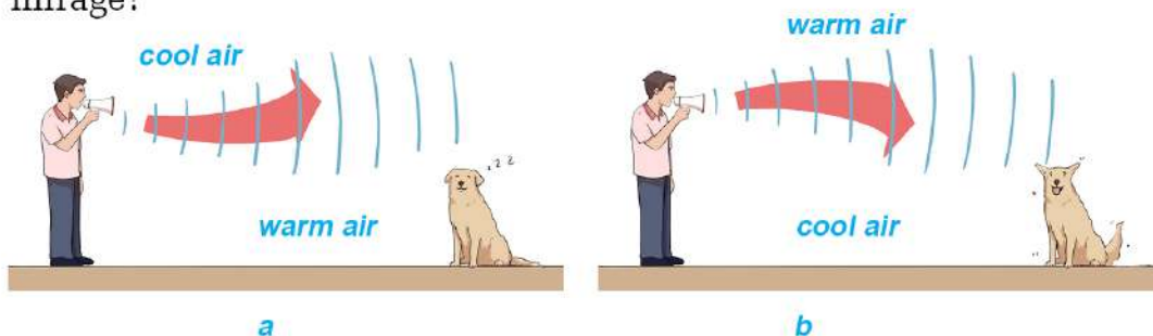
Figure 10.31 Refraction of sound
