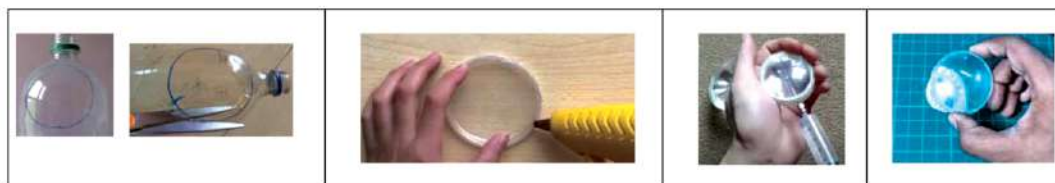
Figure 10.48 Making a hand lens
