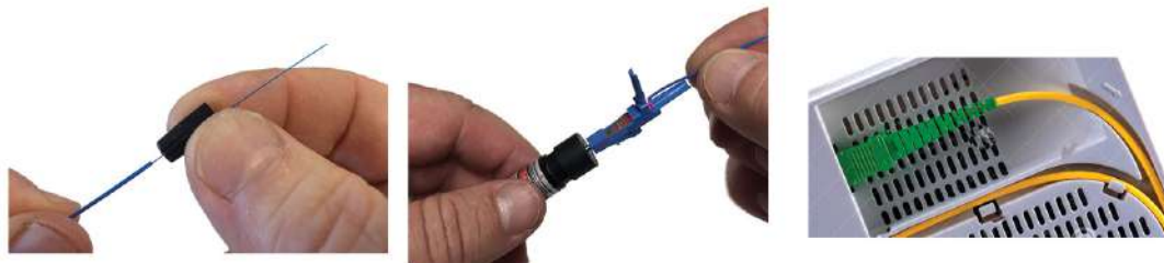
Figure 10.32 Connection of optical fibre connector in a router
