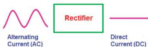
Figure 11.7 Rectifier block line graph
