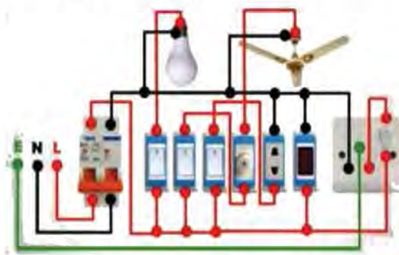
Fig 8.24 Connection of the bulbs in household electrification
