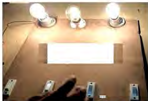
Fig 8.25 Connecting bulb to the electric circuit
