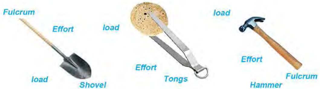
Fig 6.12 Second Class Lever
